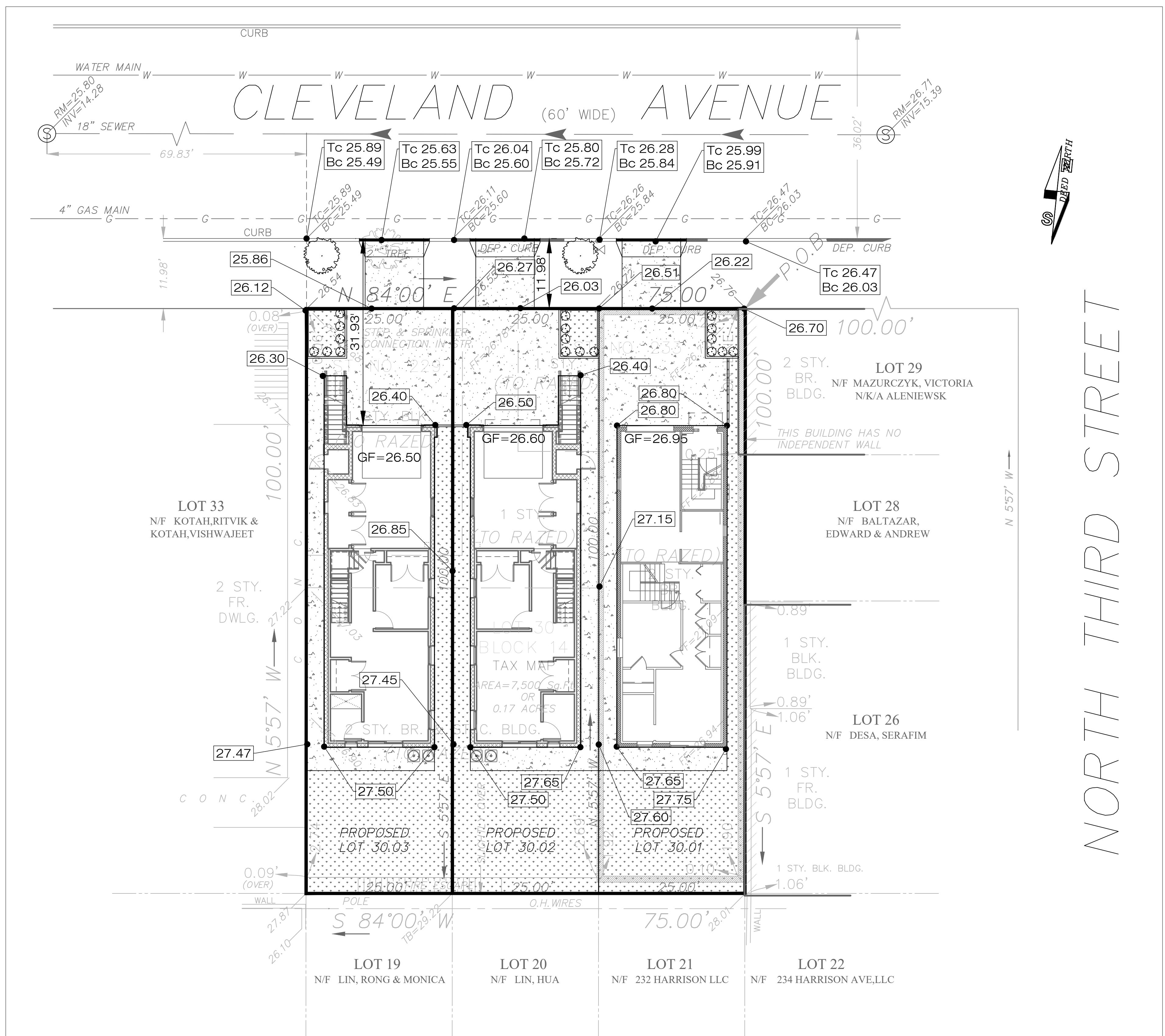
NOTE: THE EXISTING CURB AND SIDEWALK ALONG THE FRONTOAGE OF THE PROPERTY SHALL BE REPLACED PER ADA REQUIREMENTS (MAX. CROSS SLOPE @ 2%).
